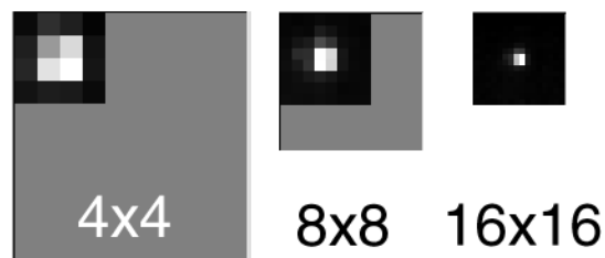
Figure 218: Different sizes of the AO track box. From left: Small, Medium, and Large.
