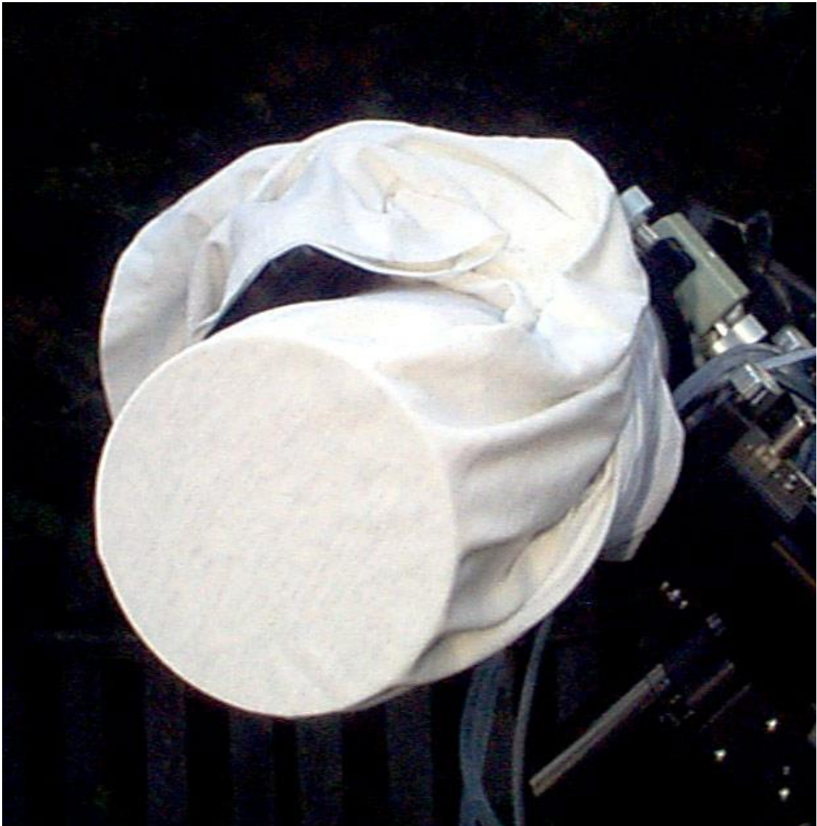
Figure 229: Using a T-shirt to take a flat in daylight. Be sure to point the scope away from bright sources of light.
