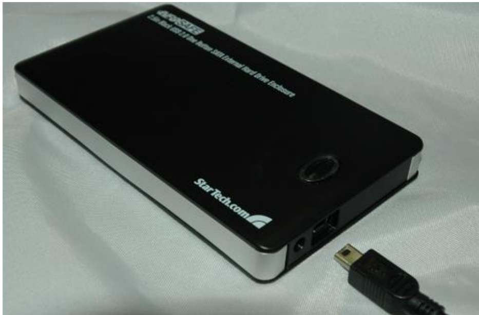
Figure 275: Plug the Mini USB end of the cable into the mini-USB port.
