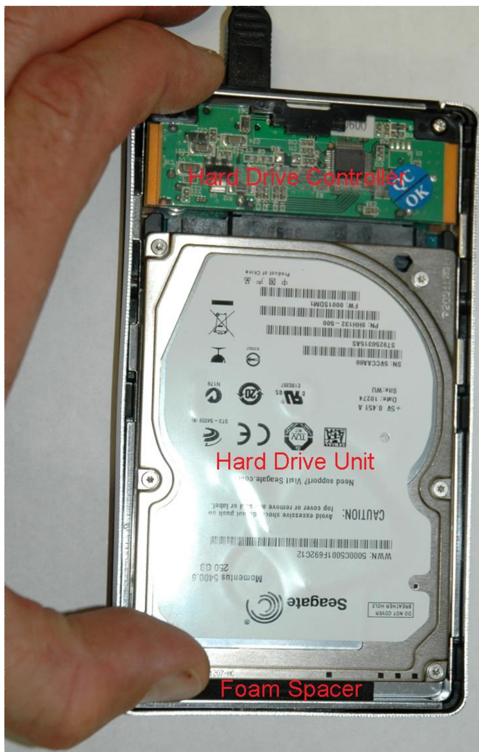
Figure 277: Finger placement to properly reseat the hard drive in the hard drive controller. (Photographer's right hand is holding the camera.)
