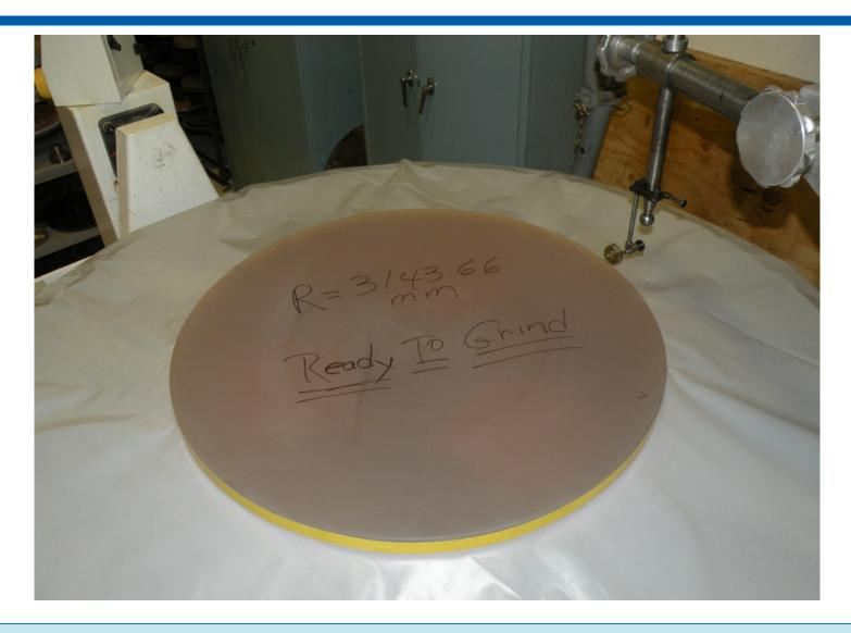
Mirror in grinding. Equipment processes up to Ø1500mm optics. Grinding curve indicated is flatter compared to final parent radius—this is intentional. Centration is critical here, and is held to about 25 microns. This photo 2/21/11.
