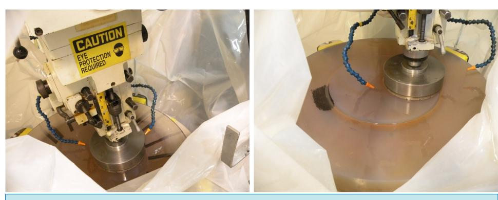
Mirror curve is generated. It is critical that mirror center thickness and orthogonality (wedge) are managed properly at this stage. Photos from about Feb 14, 2011.
