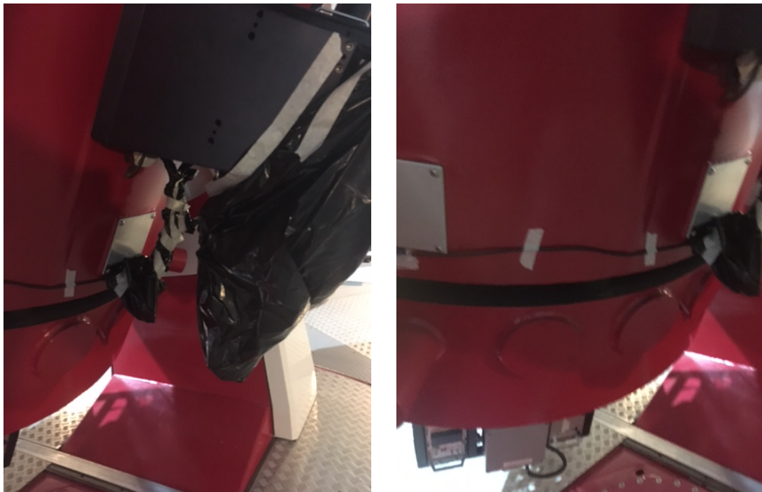
Fig. 6. Left hand panel: PISCO inside the clean rubbish bag; another bag has been used to insulate the dangling wires.
