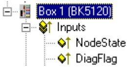
Fig. 135: Diagnosis of inputs in the TwinCAT tree
