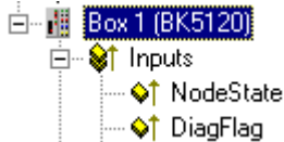
Fig. 138: TwinCAT tree: Diagnostic Inputs
