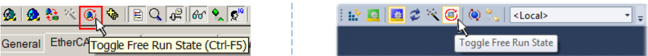
Fig. 70: TwinCAT can also be switched to this state by using a button (left: TwinCAT 2; right: TwinCAT 3)
