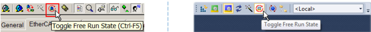
Fig. 116: TwinCAT can also be switched to this state by using a button (left: TwinCAT 2; right: TwinCAT 3)
