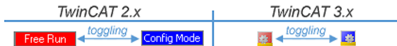
Fig. 110: Displaying of “Free Run” and “Config Mode” toggling right below in the status bar
