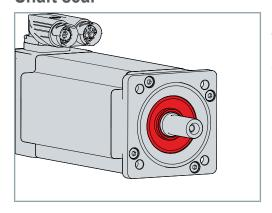
The radial shaft-sealing ring FKM is used for sealing against splash water and protects the motor shaft against dust or dirt. This increases the protection class of the shaft feed through to IP65.
