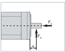
Avoid mechanically overdetermined support of the motor shaft through rigid coupling and additional external support.
