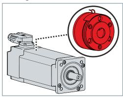
A holding brake blocks the rotor in the de-energized state. The holding brake increases the motor length and the rotor moment of inertia.
