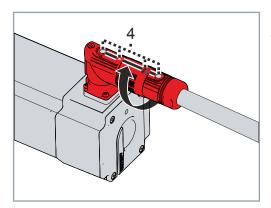
► Make sure that all markings and the lettering "open" 4 are aligned The speedtec connector is then fixed properly.
