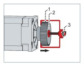
Only use backlash-free, friction-locked collets, pullers or suitable couplings for dismantling the output elements.
