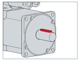
A feather key serves to transmit torques to an output element.
