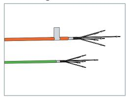
Orange power cables and green feedback cables are used for the connection between motor and servo drive.
