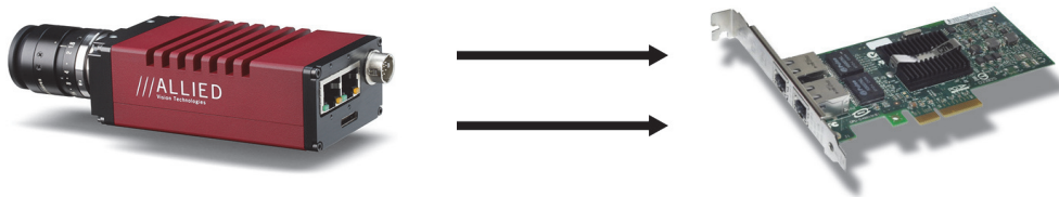
Figure 32: Prosilica GX camera network configuration using multiple Ethernet ports
