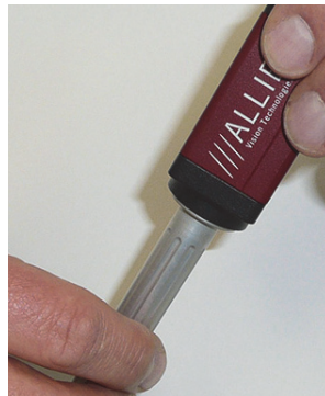
Figure 43: Removing IR cut filter/protection glass using special tool (E9020001)
