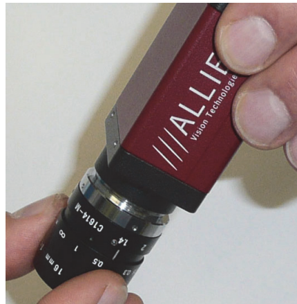
Figure 41: Camera orientation when removing lens or dust cap
