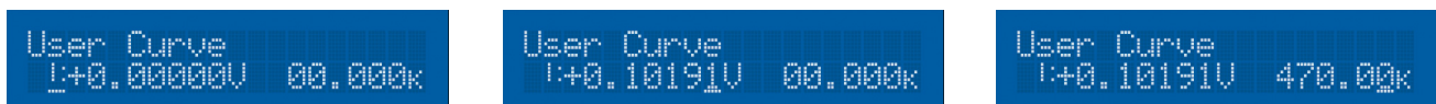
FIGURE 5-8 Left: Scroll to highlight a breakpoint number; Middle: Press the enter key to highlight the sensor value of the selected pair; Right: Press the enter key again, and the temperature value is highlighted
