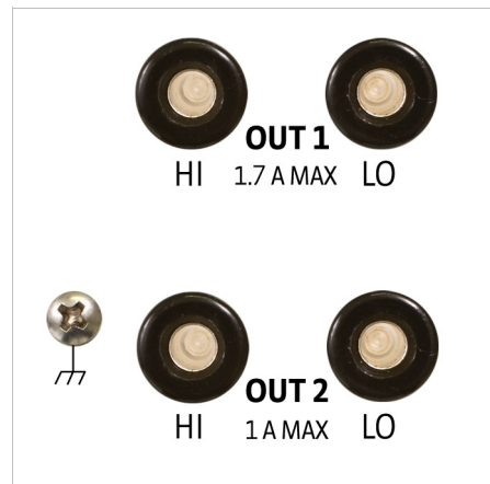
FIGURE 3-8 Rear panel showing heater output connectors
