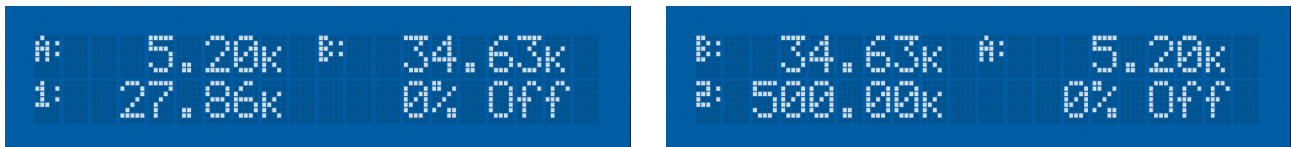
FIGURE 4-3 Left: Two Input, Loop A, showing input A and its associated information monitored; Right: Two Input, Loop B showing input B and its associated information monitored
