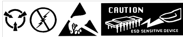
FIGURE 8-8 Symbols indicating ESD sensitivity
