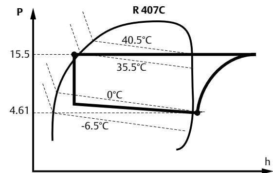
3. Multiply cooling capacity with **Kt** and **K<sub>Δp</sub>**, to find nominal capacity for Thermo®-Expansion valve.
