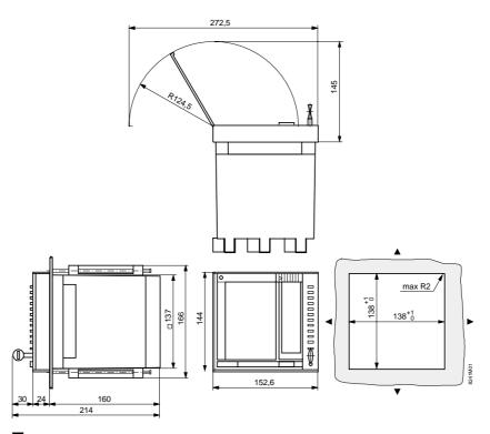
Minimum clearance to the next cut-out is 40 mm (for additional Process Units)
