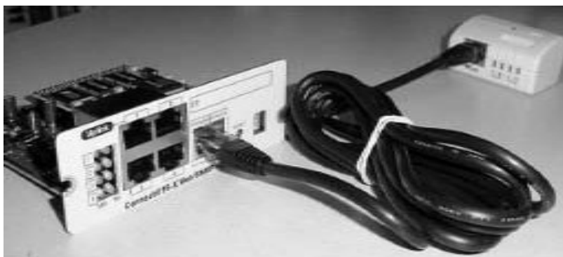
Figure 25. ConnectUPS-X Web/SNMP Module and Environmental Monitoring Probe.
